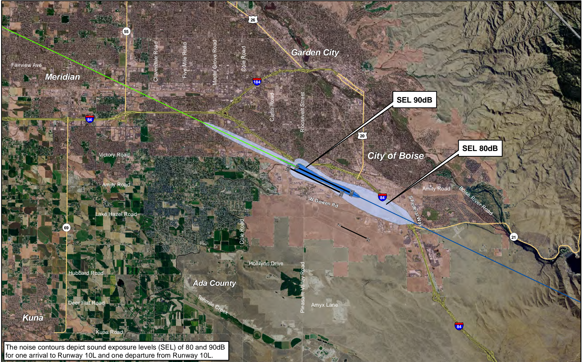
Figure B-10 Bombardier CRJ-200 Sound Exposure Level (80dB/90dB) Noise Contour
