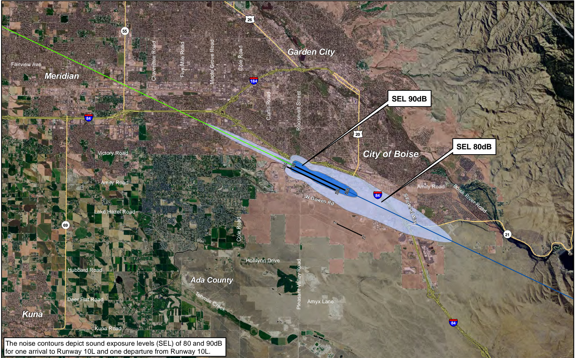
Figure B-13 Cessna 560E Sound Exposure Level (80dB/90dB) Noise Contour
